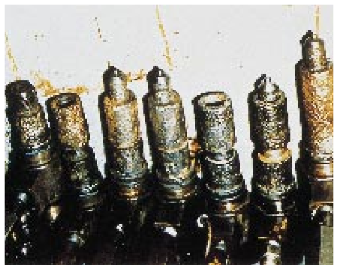
Figure 2.10 Sulphate reducing bacteria corrosion of fuel injectors
