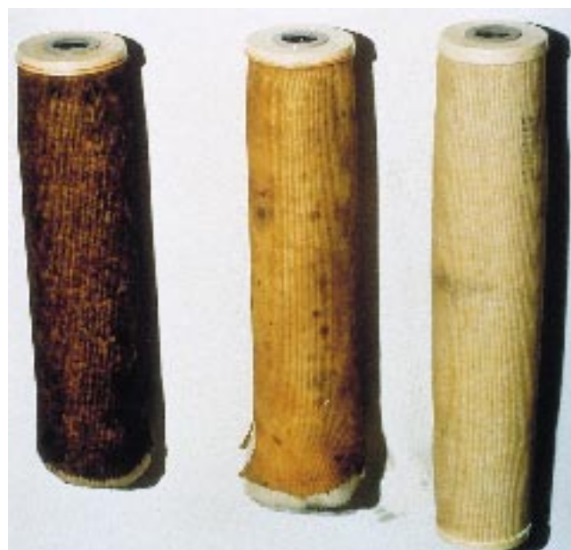
Figure 3.1 Fuel oil filter blockage from clean, initial and severely contaminated by stages
