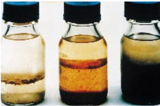
Figure 3.2 Fuel oil microbial spoilage by stages
