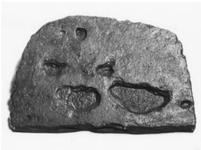
Figure 3.19 SRB corrosion of hull plates after only 9 months
